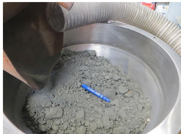
Figure 11. IPB-tailings1: picture of crushing after drying using a cone crusher (@BRGM)
