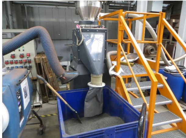
Figure 5. Cone crusher (@BRGM)
