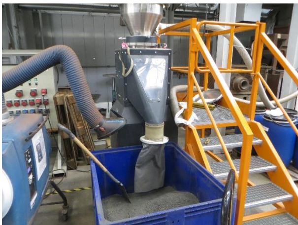
Figure 11. IPB-tailings1: picture of crushing after drying using a cone crusher (@BRGM)
