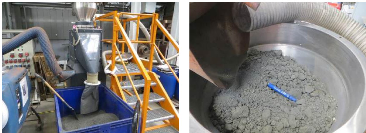
Figure 11. IPB-tailings1: picture of crushing after drying using a cone crusher (@BRGM)
