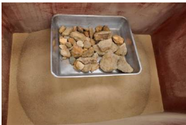
Figure 22. W-tailings: picture after screening (@BRGM)
