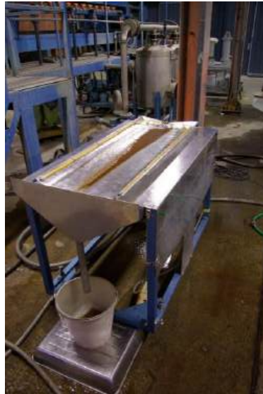
Figure 2. Mozley shaking table (@BRGM).
