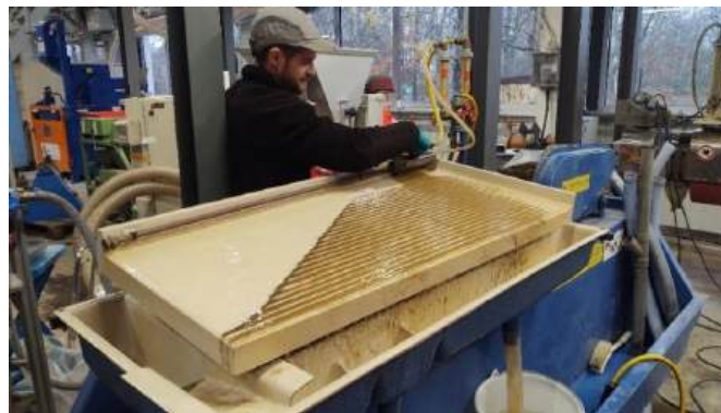
Figure 3. Wilfley shaking table (@BRGM).
