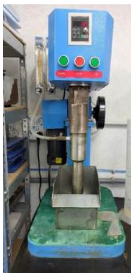
Figure 5. Flotation cell at AGQ.
